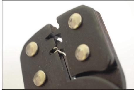
5) Insert wire into pin, with ends of conductor approximately flush with rear face of crimper jaws. (If the conductor extends too far into the pin, it can get in the way of the mating connector pins.) Then close crimping tool firmly to join pin to wire.
