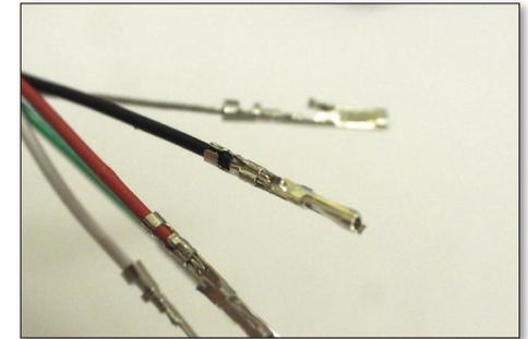
8) Insert the five pins into the connector housing, ensuring that the barb of the pin reaches the small holes in the housing so the pins can't fall out. Pins can be removed if necessary by pushing on the barb through the hole with a small tool, then pulling the pin out gently.
